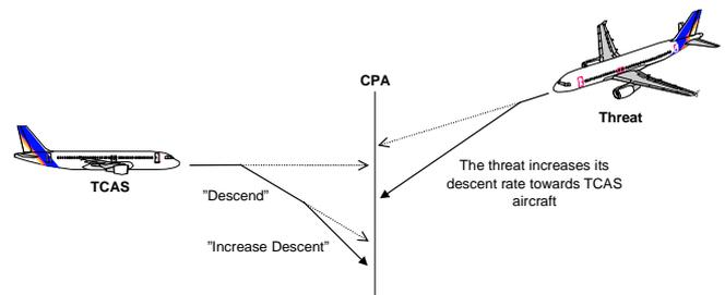
Figure 10: “ Increase-vertical-rate ” RA
