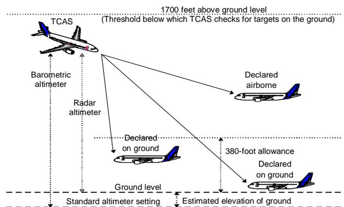
Figure 7: Target on-the-ground determination
