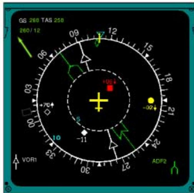
Figure 5: EFIS - Navigation Display in "ROSE" mode with traffic display
