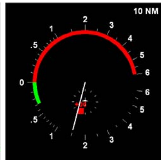
Figure 6: Weakening Level Off RA as shown on a generic IVSI display (incorporating a traffic display.)
