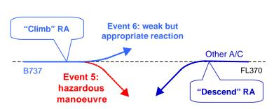
received a coordinated "Descend" RA, which was correctly followed by the pilot. The vertical separation achieved was the vertical deviation of the descending aircraft **PLUS** the 100 ft achieved by the B737.
