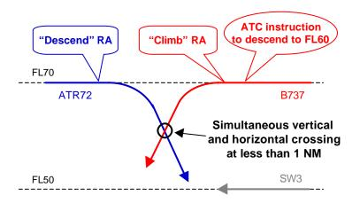
The ATR72 pilot immediately informs the controller that he has a "Descend" RA using the standard phraseology. However just after, the controller repeats to the B737 the instruction to descend to FL60 for avoiding action.
